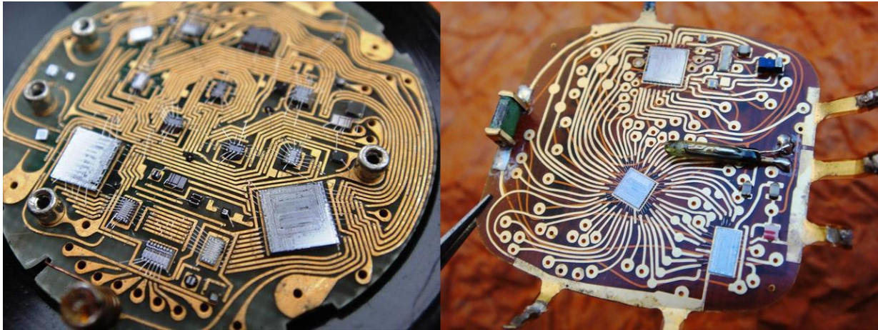
Figure 2.10 - 'Motherboards' of the Uranus (left) and a Pulsar Calculator Watch (right) [110]
