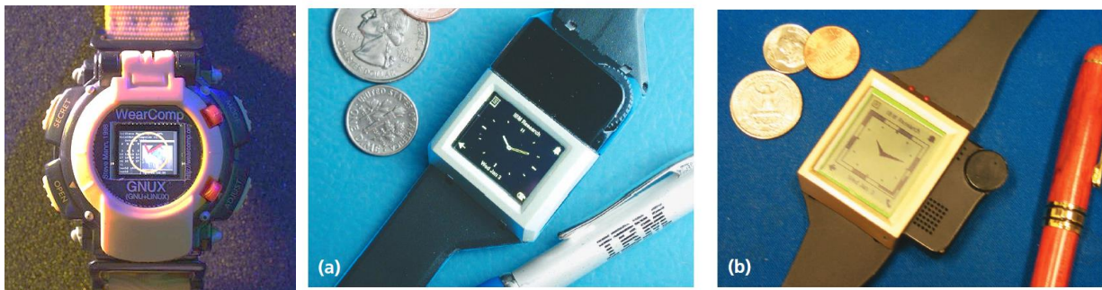
Figure 2.13 – Linux watch by Mann [126], OLED and LCD versions of Linux watch by IBM [95]
