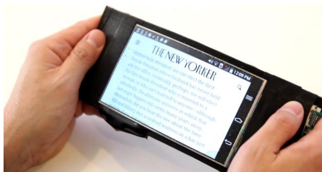
Figure 1. ReFlex, a flexible haptic smartphone.
