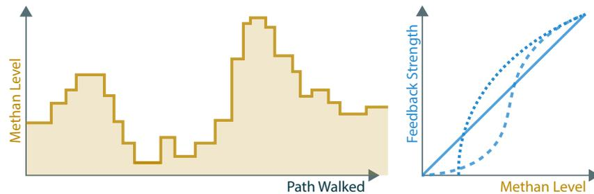
Figure 66: Interaction in the *Cognitive Band* as the user walks through Tidmarsh, the levels of methane vary (left). Based on the methane concentration the amplitude of the vibrotactile feedback is adjusted (right).
