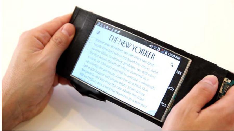
Figure 18: Reflex – a flexible, haptic smartphone.
