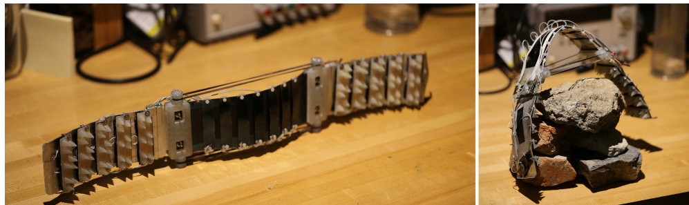
Fig. 8 Single node Grappler with a n=1 bistable elements and flat end effectors
