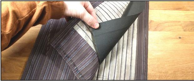
**Figure 3: Multi-layer structure of eTextile sensor: non-conductive (outside), piezo resistive (center) and conductive (in strips) materials combine to form the sensor.**
